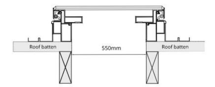
Standard installation frame opening size required: 550mm x 800mm Frameless installation frame opening size required: 480mm x 730mm
