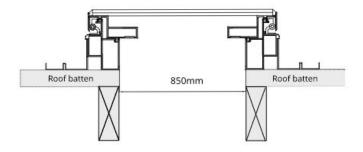
Standard installation frame opening size required: 850mm x 1100mm Frameless installation frame opening size required: 780mm x 1030mm
