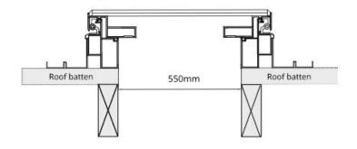
Standard installation frame opening size required: 550mm x 1100mm Frameless installation frame opening size required: 480mm x 1030mm
