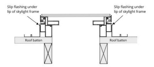
2. Next install the side flashings under the skylight lip and OVER the bottom flashing and using screws to secure it into position.
