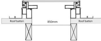
Standard installation frame opening size required: 850mm x 850mm Frameless installation frame opening size required: 780mm x 780mm
